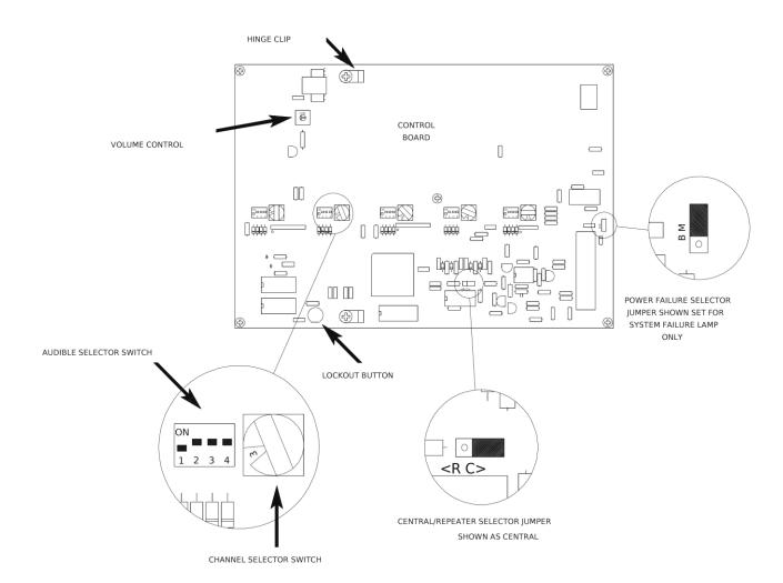
Mount the front plate and PCB onto the hinge by springing the ends of the hinge apart and fitting into the clips on the PCB. Plug the ribbon cable on the power supply into the control PCB. (it is keyed to prevent incorrect connection). Switch on the power to all
